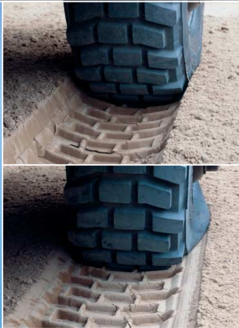
With tirecontrol, the tyre pressure can be adjusted while in motion to suit the terrain – at the push of a button
