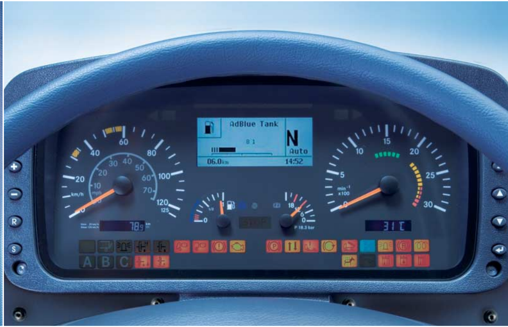
The instrument panel: clearly structured with an easy-to-operate driver information system (FIS), illuminated dials and 2 LCD multi-function displays
