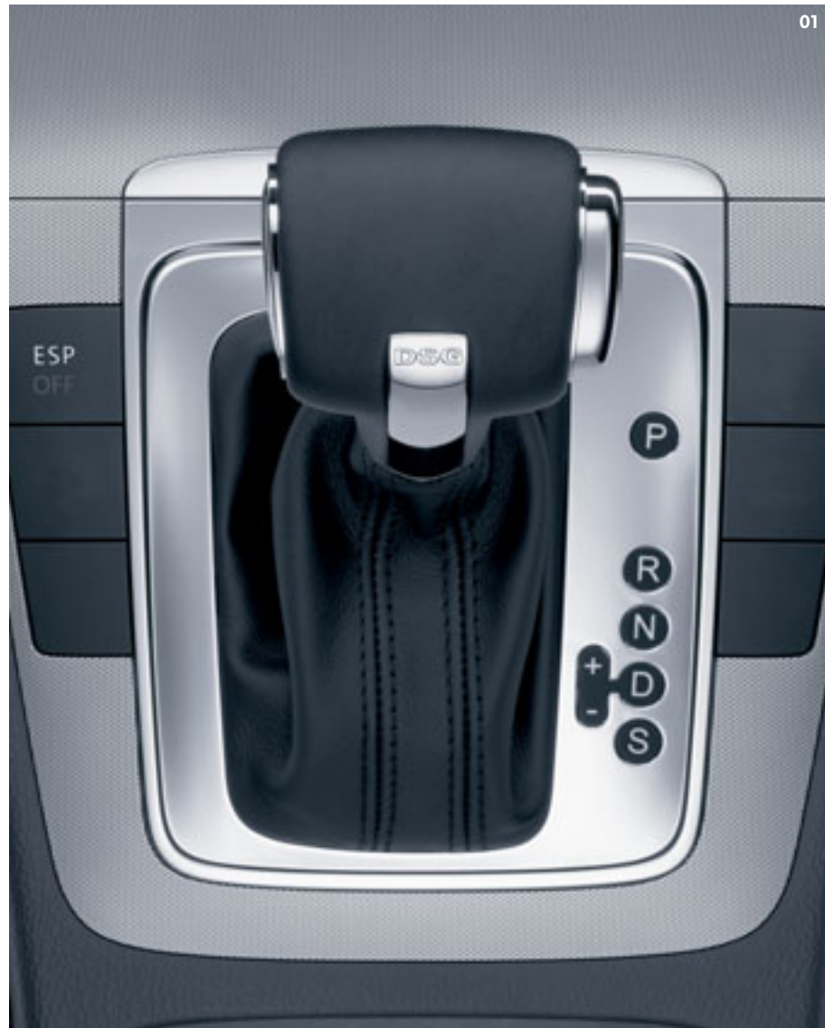
01. The DSG gearbox offers a genuine alternative to a manual gearbox because it is able to change gear faster than a manual gearbox and more smoothly than a conventional automatic.
