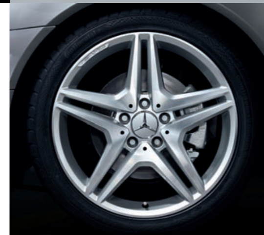
18" AMG 5-twin-spoke wheel | Style IV AMG light-alloy wheel Finish: silver, high-sheen Wheel: 7.5 J x 18 ET 37 | Tyre: 225/40 R18 Option for rear axle: Wheel: 8.5 J x 18 ET 30 | Tyre: 245/35 R18 | also available as 17" wheel | pictured on p 45 |
