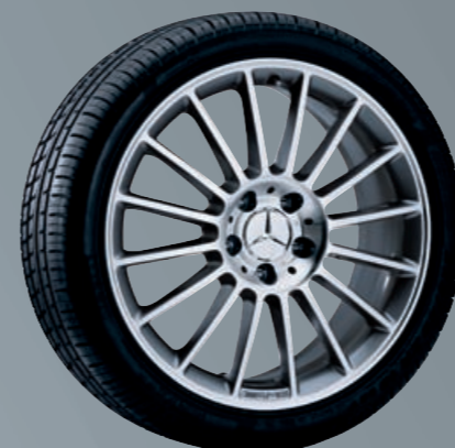
18" AMG multi-spoke wheel | Style V AMG light-alloy wheel | Finish: titanium grey, high-sheen Wheel: 7.5 J x 18 ET 37 | Tyre: 225/40 R18 Option for rear axle: Wheel: 8.5 J x 18 ET 30 | Tyre: 245/35 R18
