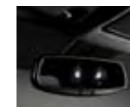
EC mirror RAV4 XT5's electrochromatic rear-view mirror cuts down headlight glare from cars behind you when driving at night.
