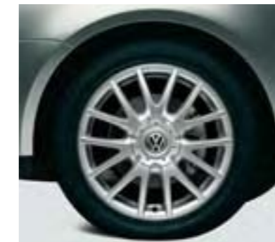
'ClassiXs' design 7J x 17 light alloy wheels with 225/45 R17 tyres. Standard on Sportline models.
