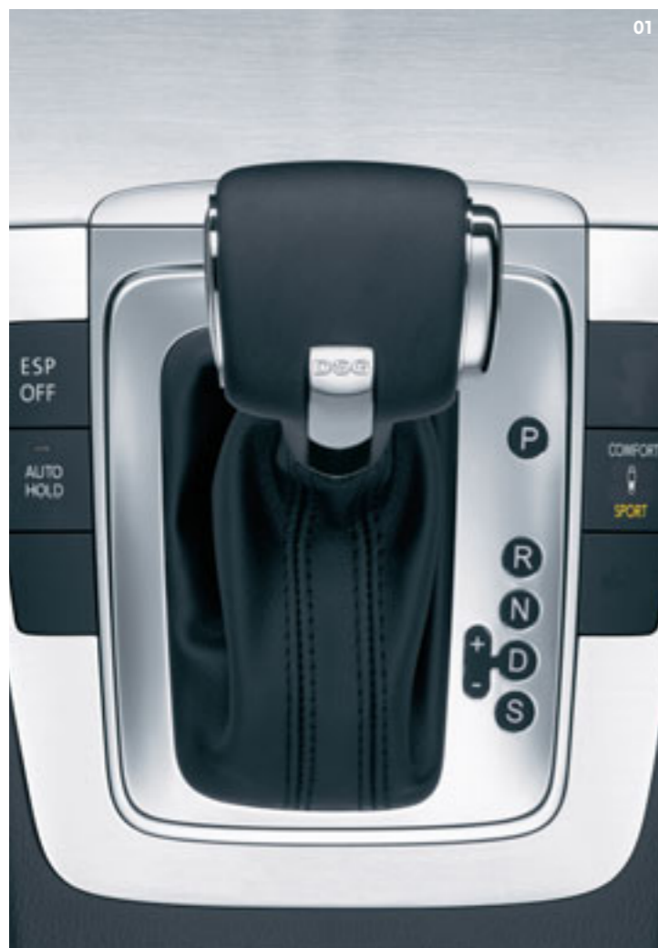
01. The DSG gearbox offers a genuine alternative to a manual gearbox because it is able to change gear faster than a manual gearbox and more smoothly than a conventional automatic. On SEL V6 4MOTION models ACC (Adaptive Chassis Control) is standard.
