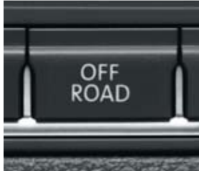
Control: The off-road mode includes hill descent assist and ABS adjusted to suit loose ground.
