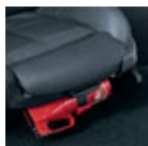
Powder-type fire extinguisher
