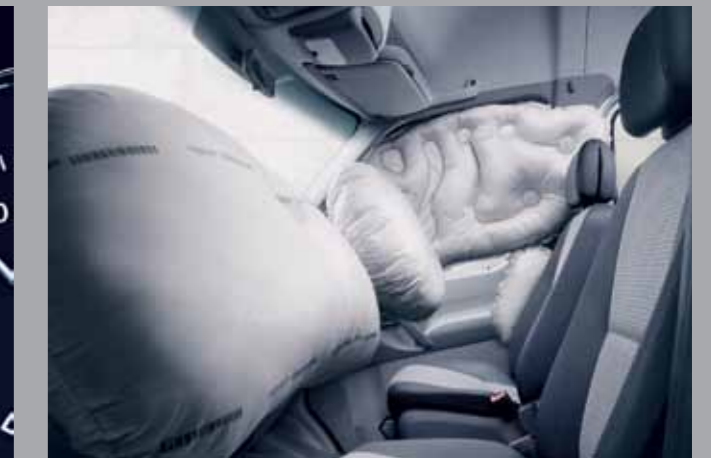
Air bags – optional window and even thorax bags can provide additional safety to driver and front-seat passenger airbags (shown activated for illustrative purposes only).
