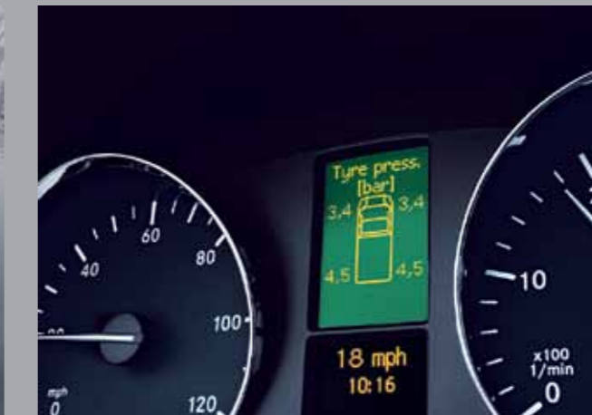
Optional automatic tyre pressure monitoring provides advance warning to the driver of possible imminent tyre failure.
