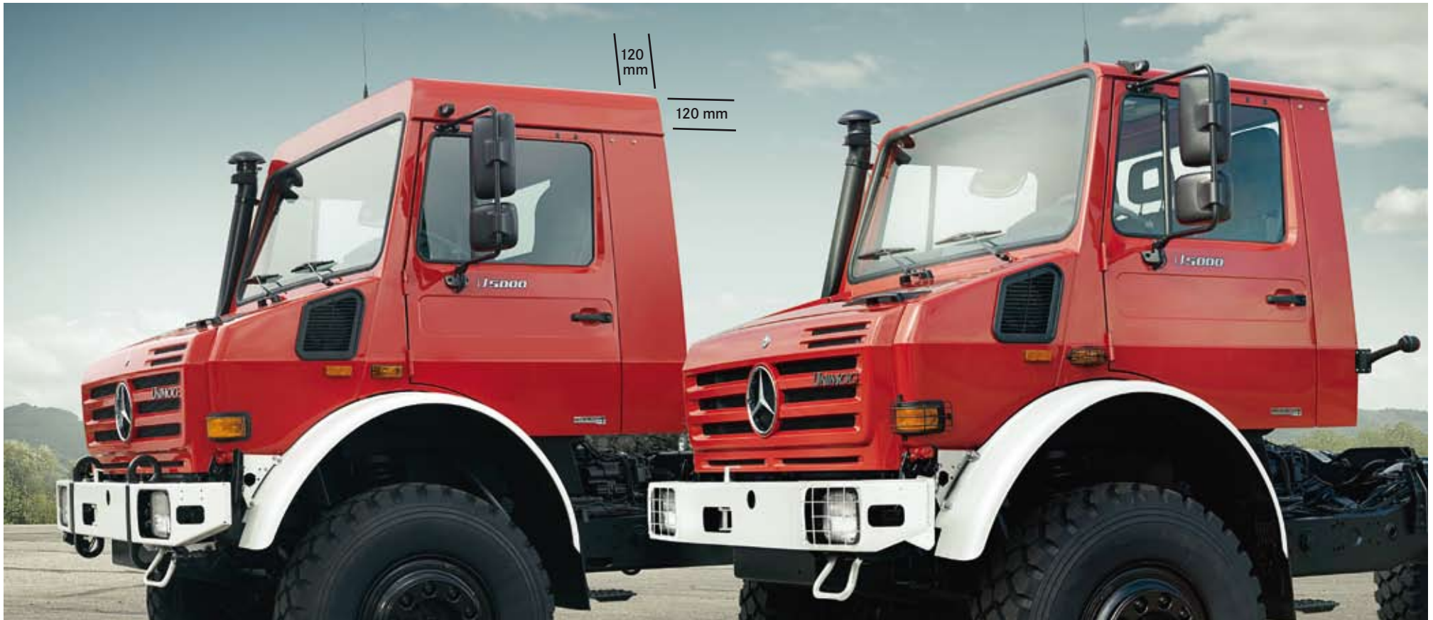
Direct comparison: the optional enlarged cab (left) and the standard cab (right)
