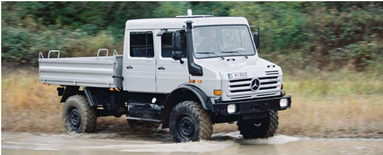
Spacious crewcab accommodates up to seven persons, or, as option, is available with four air-sprung individual seats
