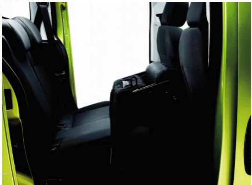
The rear seats can be folded in a 2/3 1/3 configuration, creating a load space of 884 litres with all the rear seats folded flat.
