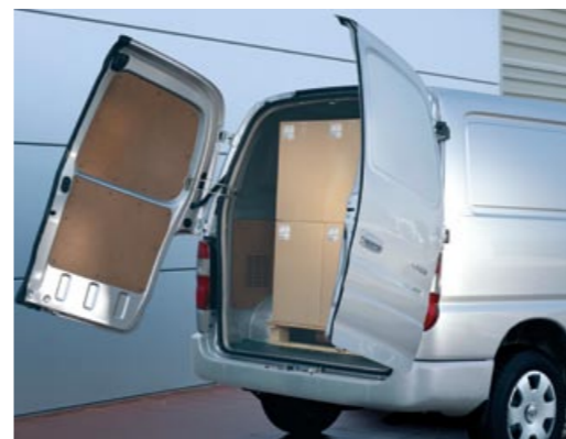
Rear door options Hiace vans are available with wide-opening blind, double rear doors or a single, tailgate-style rear door with window.
