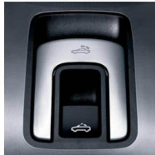
Switches for controlling the automatic CSC roof system and slide/tilt glass sunroof are located within the centre console.
