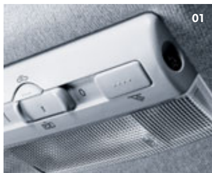
01 The optional alarm with interior protection has a monitor that detects movement in the car and, if appropriate, triggers the alarm.
