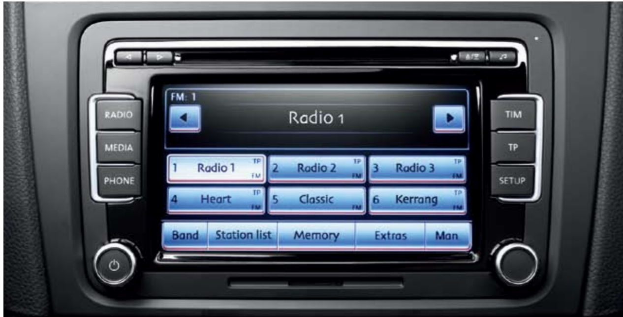
The optional RCD 510 touch-screen radio/dash-mounted MP3 compatible six CD autochanger features a large 6½ inch colour display, with intuitive menu navigation and touch-screen operation. It also features an AUX-in socket for connection to an external multimedia source (e.g. iPod or MP3 player) and an SD memory card slot.
