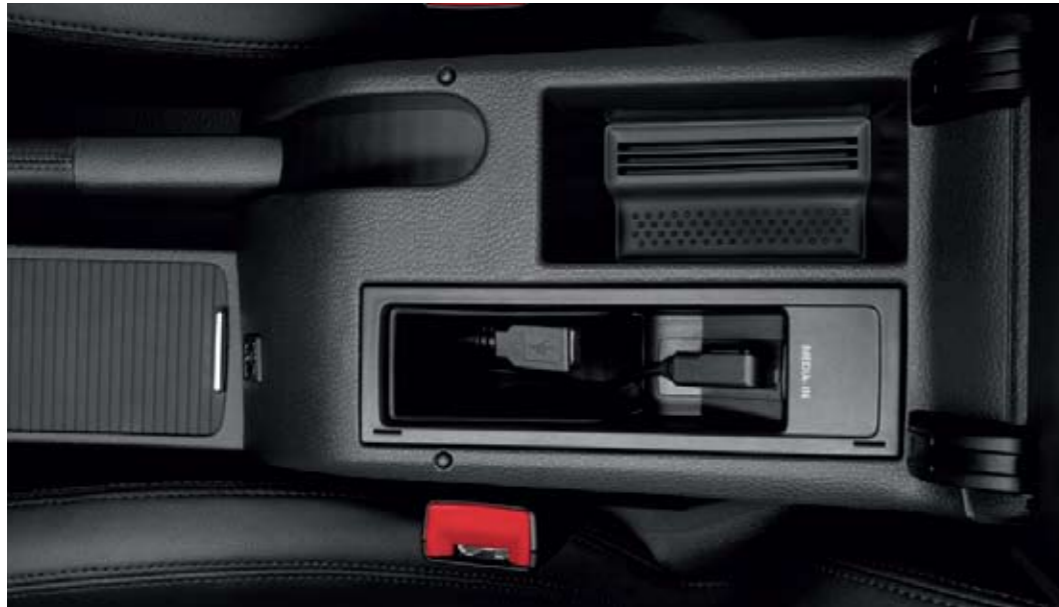
The Multi Device Interface (MDI) with iPod and USB cables enables you to connect and charge a compatible device, while track selection is viewed and selected via the vehicle's radio system.
