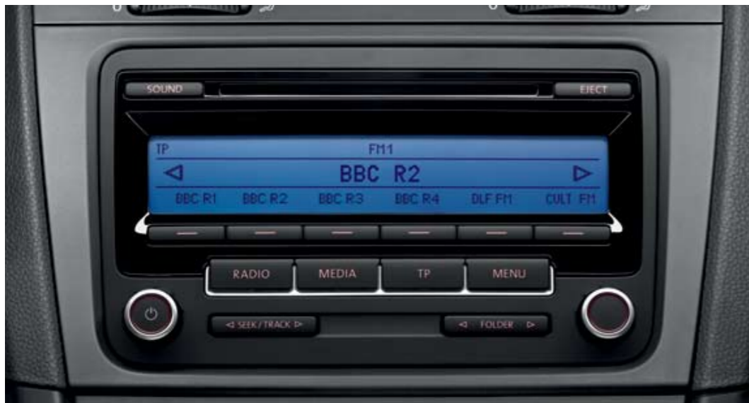
The RCD 310 radio/MP3 compatible CD player features eight speakers with an output of 4 x 20 watts and its large screen clearly displays radio station choices or the track listings of a compatible device connected to the Multi Device Interface (MDI).
