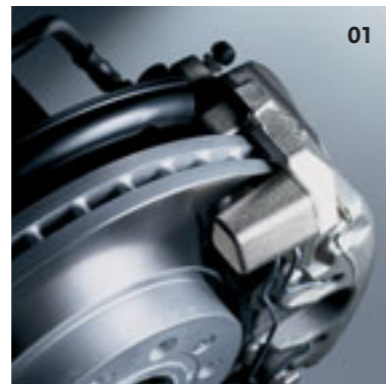
01 Disc brakes all round, the front with interior ventilation, ensure optimum brake power at anytime.
