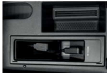
The front centre armrest features both a Multi Device Interface (MDI) and an AUX-in socket and with the facility to connect, charge and store a compatible iPod or USB device. The rear passengers also benefit from two rear air vents and two cup holders.
