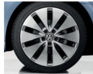
'Bilbao' 7½J x 18 light alloy wheels with 225/40 R18 tyres. Optional on GT models.
