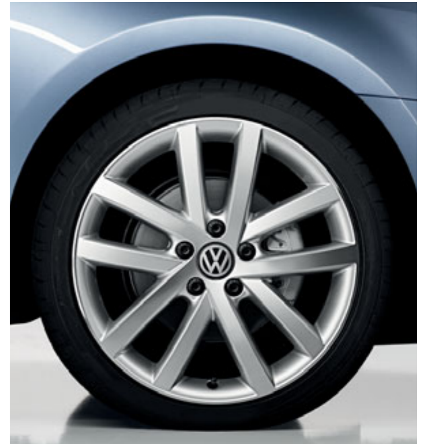
'Vancouver' 7½J x 18 light alloy wheels with 225/40 R18 tyres. Optional on GT models.
