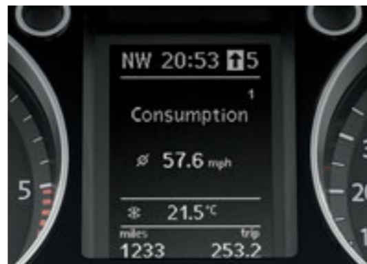
The multifunction computer (Highline) includes visual gear change recommendation for optimum fuel consumption. Standard on BlueMotion 2 models.
