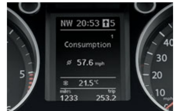
The multifunction computer (Highline) includes visual gear change recommendation for optimum fuel consumption. Standard on BlueMotion 2 models.
