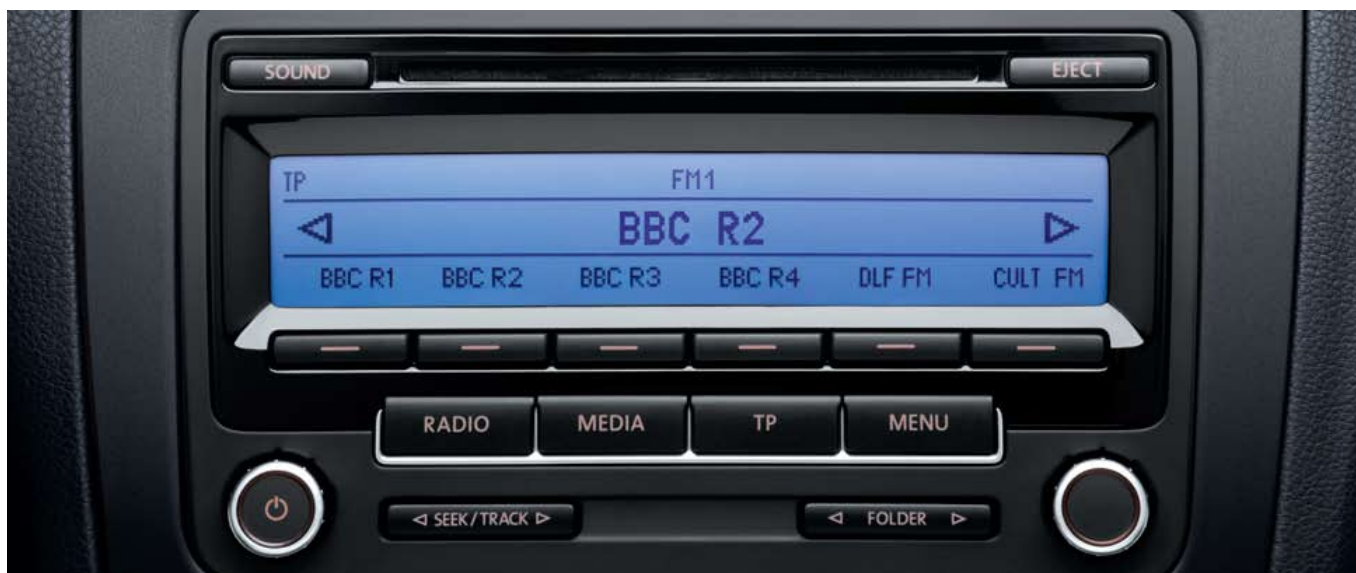
The RCD 310 radio/MP3 compatible CD player features six speakers and its large screen clearly displays radio station choices or the track listings of a compatible device connected to the Multi Device Interface (MDI).
