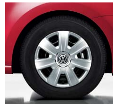
14 inch steel wheels with 175/70 R14 tyres and full size wheel trims feature a robust seven spoke design, adding a sporty touch. Standard on S models.
