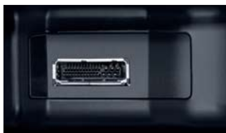
The Multi Device Interface (MDI) allows you to connect to an external multimedia source, such as USB or iPod, which you can operate via the vehicle's radio or optional navigation/radio system.
