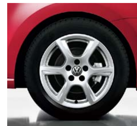
'Cadiz' 6J x 15 alloy wheels with 195/55 R15 tyres and anti-theft wheel bolts add a particularly dynamic look, emphasising the Polo's sporty aesthetics. Standard on Moda and optional on S models.
