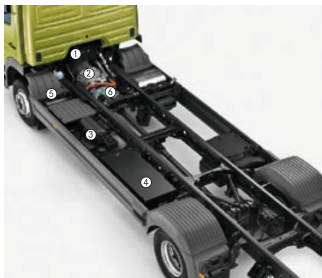
The key components of the Atego BlueTec® Hybrid drive system at a glance: 1. Diesel engine 2. Electric motor/alternator 3. Inverter (below equipment carrier) 4. Lithium-ion battery 5. Hybrid cooling system for electric motor/alternator and inverter 6. Automated transmission with Telligent® automatic gearshift
