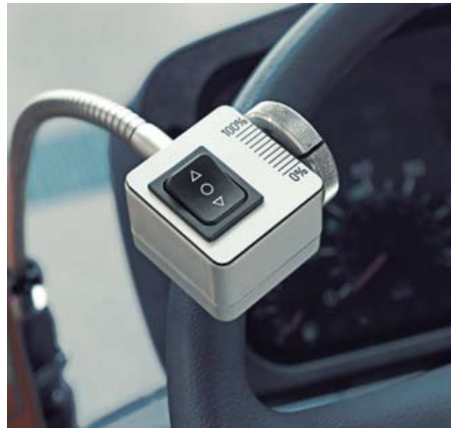
Hydrostatic drive can be regulated individually using manual shift
