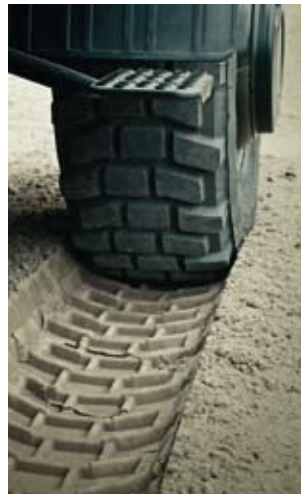
With Tirecontrol, the tyre pressure can be regulated while on the move
