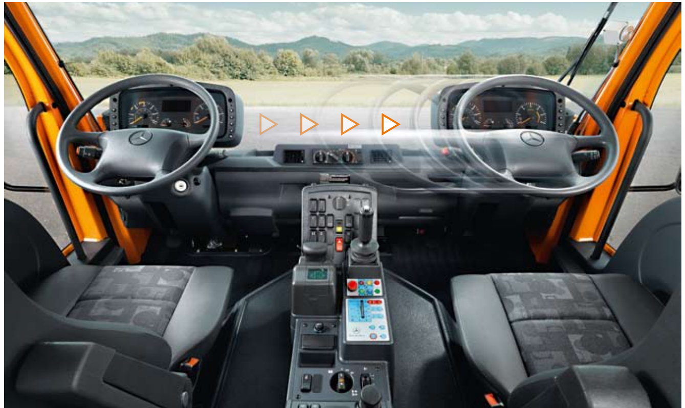
The VarioPilot® transferable steering can be slid from the left to the right side of the cab in an instant – ideal for safe and convenient one person operation
