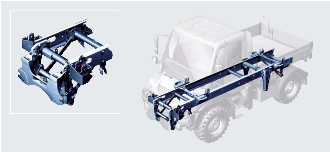
A robust, continuous ladder-type frame with integrated fastening points make direct implement mounting simple and inexpensive
