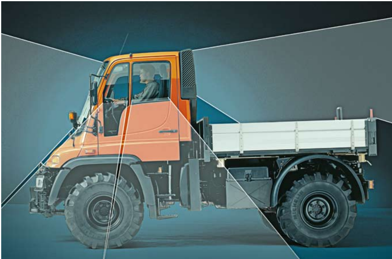
The deep windscreen, deep-drawn side windows and the large rear window offer excellent and safer view to all sides
