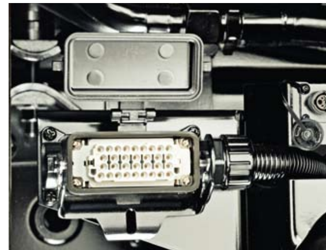
The socket to supply electricity for implements. Current collection up to 40 A
