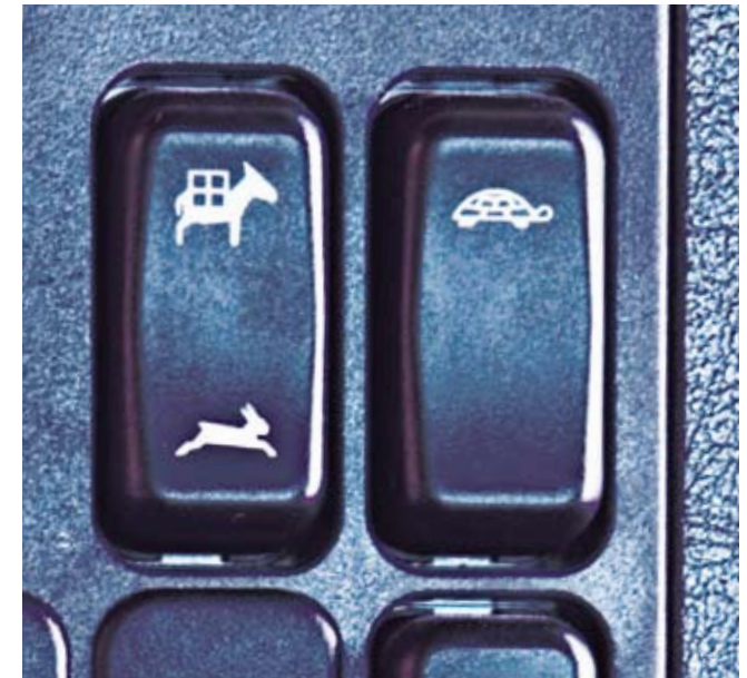
Rocker switch in the centre console for the basic, working and crawler gears
