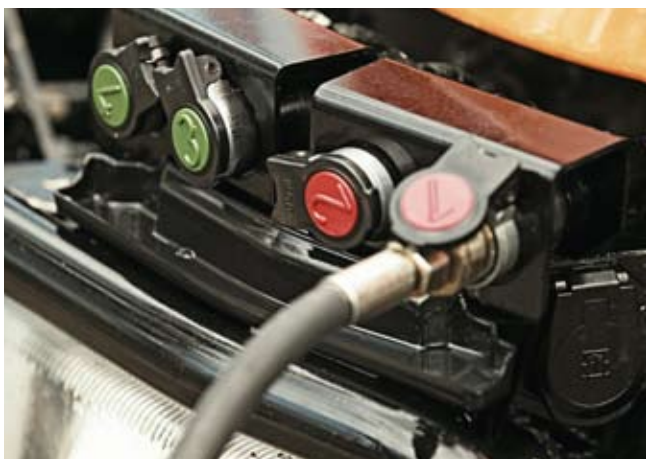
The power hydraulic connections are coded by colour and number – perfect for connecting implements quickly and without any error
