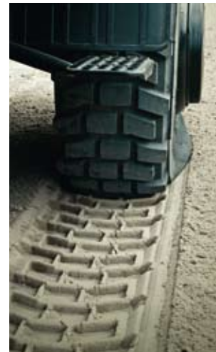
With Tirecontrol, the tyre pressure can be regulated while on the move
