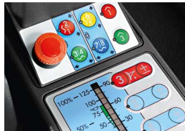
The key pad shows the valves and connections arranged by colour and number
