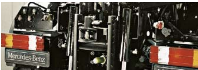
Front PTO for implements with a high output. Retrofit: rear PTO in standard configuration
