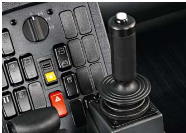
The gate-guided joystick gives you simple, convenient control over all implement movements
