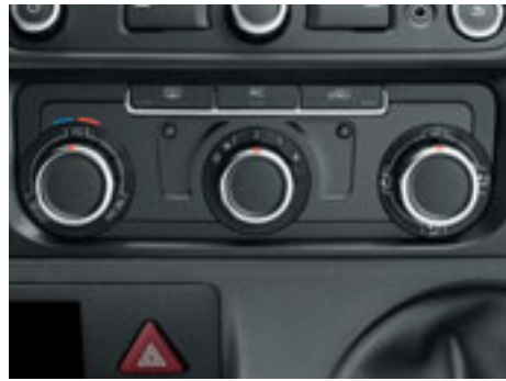
Air conditioning - 'Climatic'.
