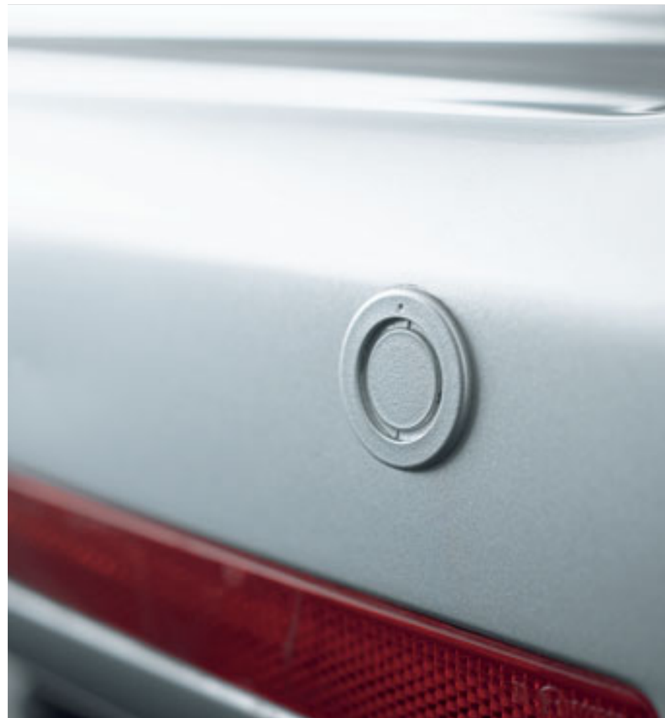
Reversing aid kit. This kit includes four sensors which can be painted to match the body colour of your vehicle.
