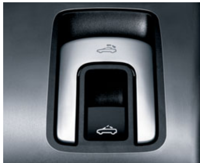
Switches for controlling the automatic CSC roof system and slide/tilt glass sunroof are located within the centre console.
