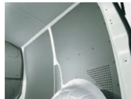
Full-height load side lining.
