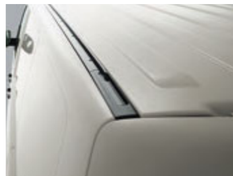
Roof load rack preparation.
