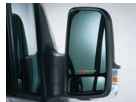
Electric mirrors. Image shows Parking sensors display.
