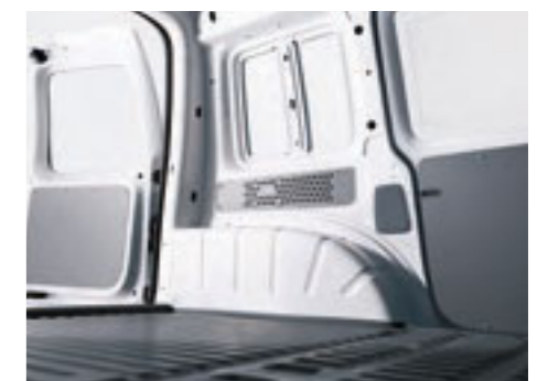
Load side lining.
