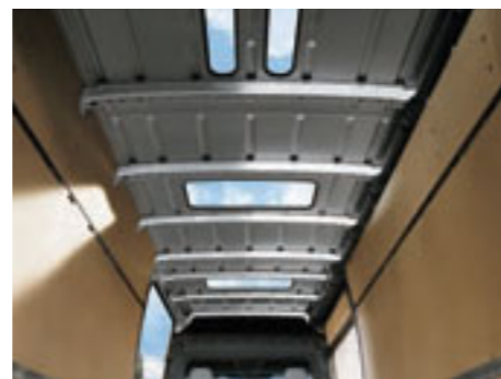
Skylights in load compartment.
