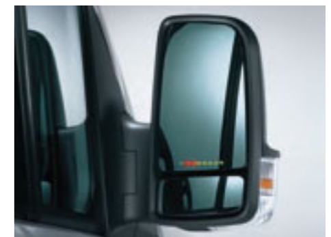
Electric mirrors. Image shows Parking sensors display.
