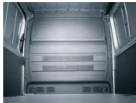
Full height steel bulkhead.
