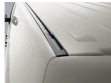
Roof load rack preparation.
