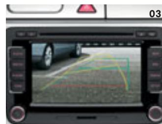
03 Park Assist, parking sensors and rear-view camera.
