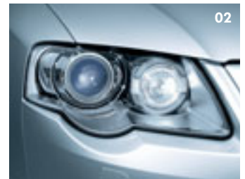
02 Gas discharge (Bi-Xenon) dipped and main beam headlights.
