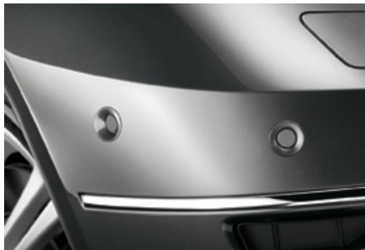
Proximity sensors in the front and rear bumpers monitor the distance to the nearest vehicle or obstacle
