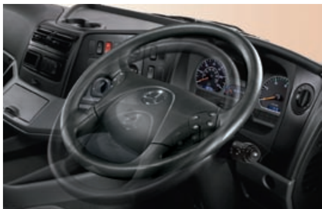
Standard equipment for the Axor includes a multifunction steering wheel that is adjustable for height and reach, including buttons for controlling the driver information system, radio and telephone, for example. The multifunction steering wheel is also optionally available in high-grade leather
