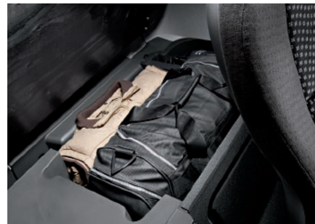
Beneath the standard lower bed there are three large stowage compartments with a total capacity of around 300 l, of which the centre compartment can be fitted with a refrigerator. As an alternative to the lower bed, a folding bed is available for the extended day cab
