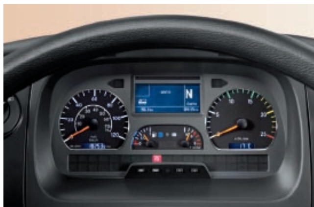
The instrument cluster trimmed with chrome rings and featuring optimised menus includes a graphics-capable display, which indicates important information about the vehicle's operating status, for example. If a manual gearshift is specified, a variable, green rev counter range is integrated as standard to help reduce diesel consumption
