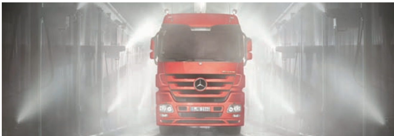
Accelerated weathering tests: during the dynamic corrosion test, the truck is subjected to extreme climatic conditions in the salt spray chamber and climate chamber for a period of several months. To test the quality of the corrosion protection for the vehicle as a whole, the truck also endures long test stretches on rutted roads, motorways, gravelled and muddy tracks
