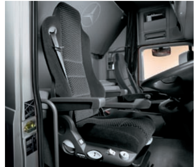
The optionally available comfort suspension seat ensures a relaxed and safe ride thanks to its versatile adjustment possibilities, such as lumbar support, lateral contour support and seat heating
