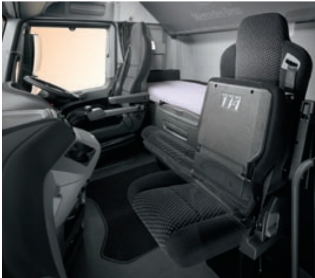
Standard: the multifunctional seat creates more space on the co-driver's side in a trice. This is because both the seat surface and the backrest can be folded, allowing a flexible and practical use of space
