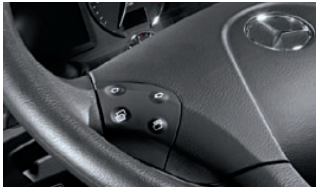
The telephone, radio and driver information system can be operated using the keys on the multifunction steering wheel, which is also available in fine leather. It can also be used to access diagnostic functions and various onboard settings – from an alarm clock to an auxiliary heater
