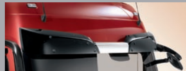
The sun visor, which is standard, improves visibility and safety. Its central stainless steel panel also accentuates the striking appearance of the Actros
