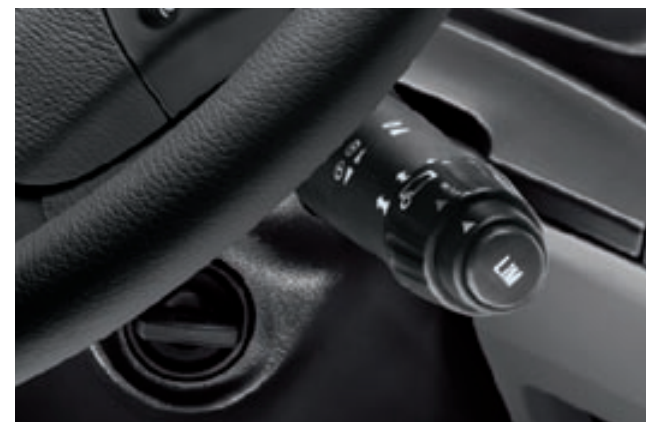
The standard-specification drive and braking cruise control function makes the driver's job easier: it combines the “Accelerate” and “Brake” functions in a single functional unit
