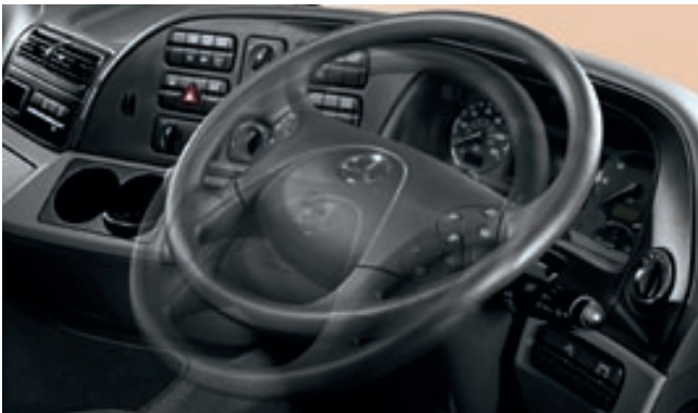
In conjunction with the driver's seat, the steering wheel adjustment range of up to 66 mm for height and from 10° to 42° for rake ensures optimal driving comfort. In addition, the 10° parking position allows easier access and egress for the driver together with excellent cross-cab access
