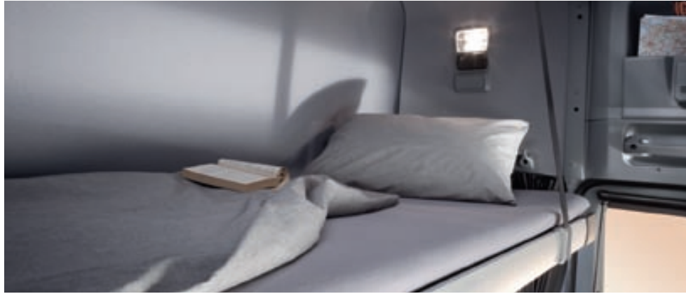
The 202x80 cm upper comfort bed (standard in sleeper cabs and the MegaSpace cab) justifies its name in every respect, as the angle of the bed surface can be variably adjusted to suit uneven ground, for example – either for sleeping or if used as a stowage area
