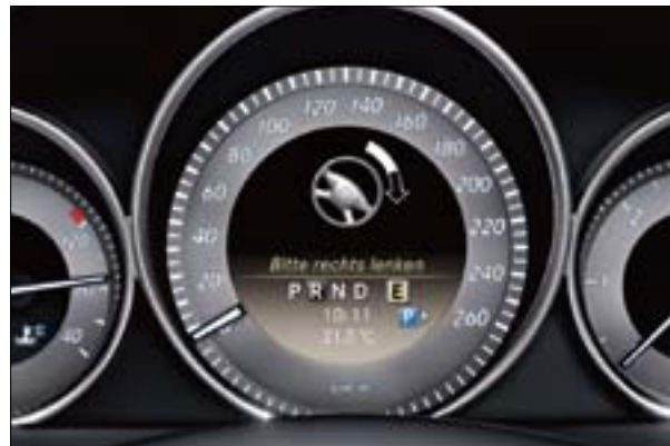
With Advanced Parking Guidance, information on the parking manoeuvre is displayed in the instrument panel
