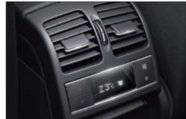
A separate control unit enables those in the rear to set their own temperature settings and blower speed
