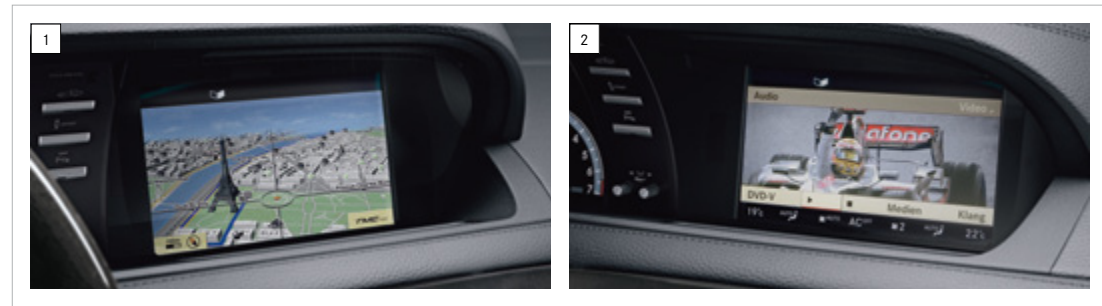
SplitView enables the screen to simultaneously display different images for the driver (1) and the front seat passenger (2)
