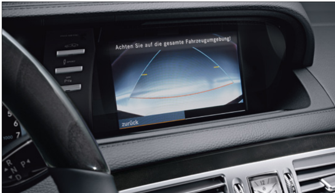
The reversing camera's wide-angle lens enables you to see what's immediately behind the car
