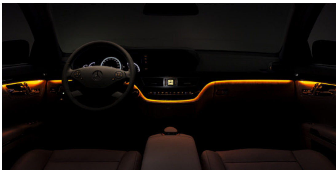
The ambient interior lighting comprises a narrow band of LEDs running around the doors and dashboard. It is dimmable and offers a choice of three colour settings
