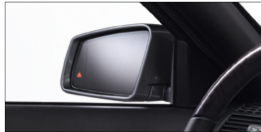
Active Blind Spot Assist warns the driver of potentially dangerous lane changes
