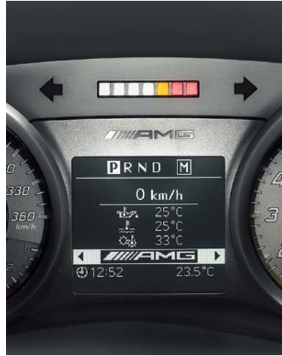
AMG instrument cluster with 7-LED upshift indicator in manual mode
