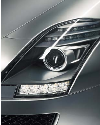
Bi-xenon front headlamps with integrated LED daytime driving lights
