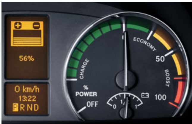
While on the move the power display shows how much energy is used or – on every application of the brakes or during overrun how much is recovered. The battery charge indicator details the available energy reserves
