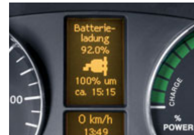
Charge indicator. By means of the on-board computer the charge level of the high-voltage battery can be ascertained at any time
