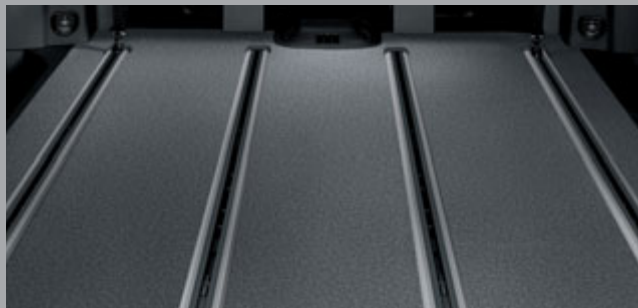
Optional seat rail system with quick-release fastener. The seat rows can be moved in 25 mm steps, enabling variable seat row spacing and arrangements, such as face to face seating to facilitate conversation during journeys
