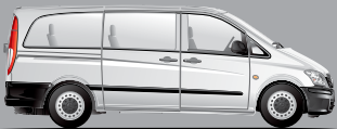
Vito Long: short wheelbase, vehicle length: 5008 mm, with normal-height or high roof
