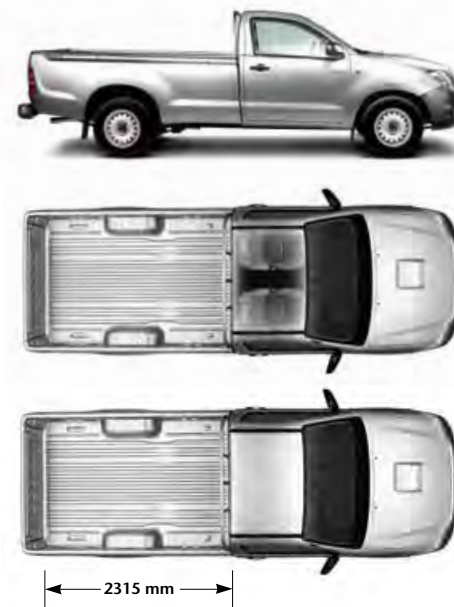
Hilux Single Cab can take a maximum payload of 860 kg and has a deck length of 2315 mm.
