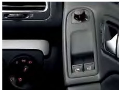
Controls for the electric front windows, including one-touch opening and closing facility, and the electrically heated and adjustable door mirror switch are conveniently located in the driver's door.
