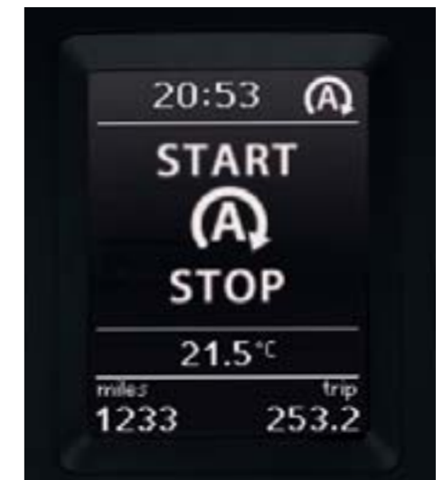
The Start/Stop function momentarily switches off the engine when the vehicle is stationary, in neutral and the clutch disengaged. This is notified to the driver with the 'Start Stop' symbol displayed on the multifunction computer (Highline).
