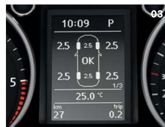
03 Tyre pressure monitoring system, electronic.
