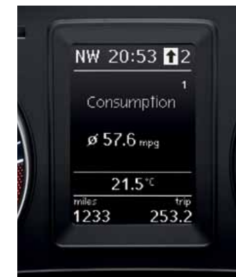
A multifunction computer (Highline) with visual gear change recommendation for optimum fuel consumption – indicates when you should change gears to drive more economically.
