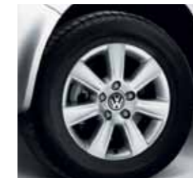
16" Cartagena alloys 6.5J x 16 alloy wheels fitted with 215/65 R16 tyres.
