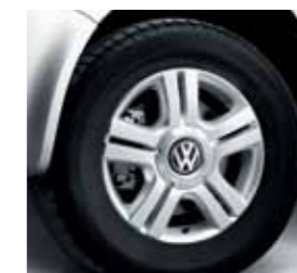
16" Los Angeles alloys 7J x 16 alloy wheels fitted with 235/60 R16 tyres (not available on 114PS BlueMotion Technology model)
