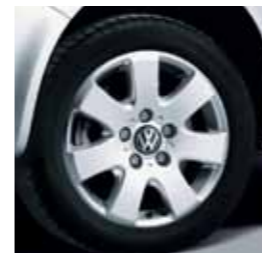
16" Miyato alloys 6.5J x 16 alloy wheels fitted with 215/65 R16 tyres.
