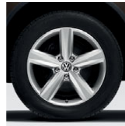
'Girona' 9J x 19 inch alloy wheels with 265/50 R19 tyres add a touch of real style. Optional on all models except Altitude V8. No cost option on Hybrid models.
