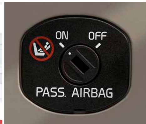
Passenger airbag cut-off switch
