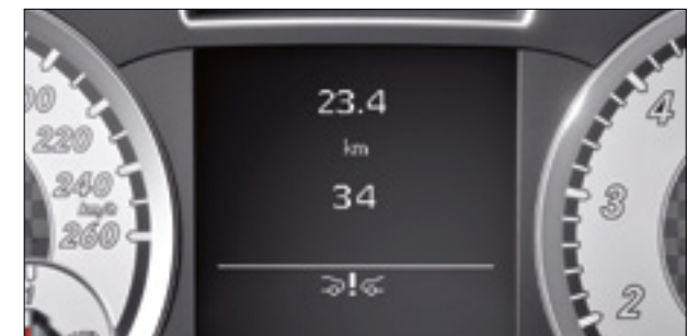
Collision Prevention Assist can warn you if it detects you come too close to the vehicle or object in front
