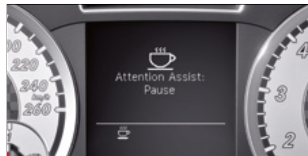
If it detects signs of tiredness or inattentiveness, Attention Assist recommends taking a break
