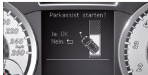
Active Park Assist displays the status of the parking manoeuvre in the instrument panel
