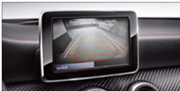
With the reversing camera, the COMAND Online display shows you what's immediately behind the car when manoeuvring
