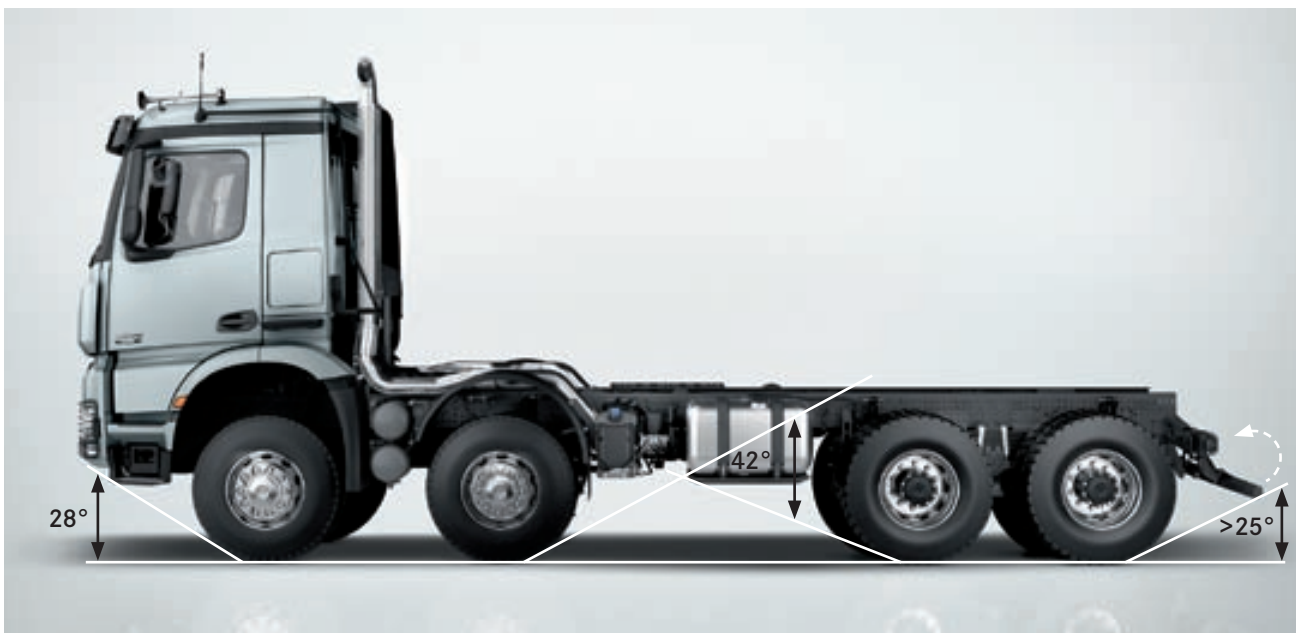
Ground clearance on all-wheel drive dump trucks. More ground clearance, improved breakover angle and greater angle of approach/departure – the Arocs all-wheel drive dump trucks display their true strengths above all away from surfaced roads and wherever uncompromising off-road capability is called for
