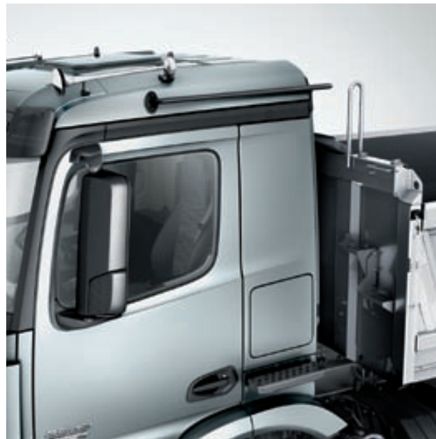
Handrail on the roof. Available on request for all Arocs cabs, the handrail on the roof makes taking a scrutinising look into the recess easier and safer. A secure footing is also ensured by the step which is also included with it and which, depending on the cab variant, is integrated into the sidewall or attached to the rear panel
