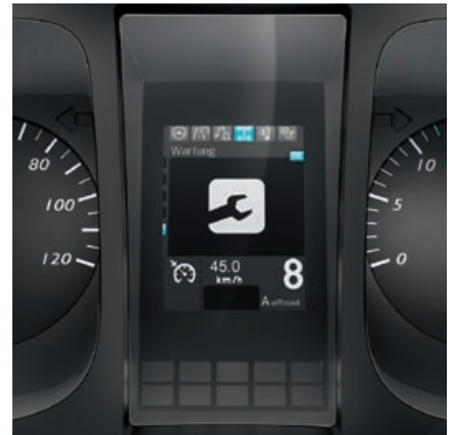
Individual maintenance intervals. The electronic maintenance system in the Arocs is guided by the actual wear rather than the mileage – meaning that the reserve power in the fuels and lubricants can be used to the full and maintenance work sensibly combined
