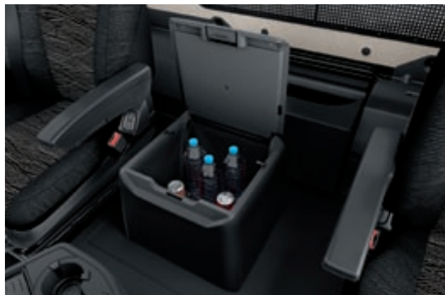
High stowage compartment on the engine tunnel. Available on request for cabs with an engine tunnel, the high stowage box makes it easy to keep everything neat and tidy – it includes an integral refuse container and can be closed with a lid. Alternatively the high stowage compartment can also be configured as a coolbox with a capacity of approximately 15 l
