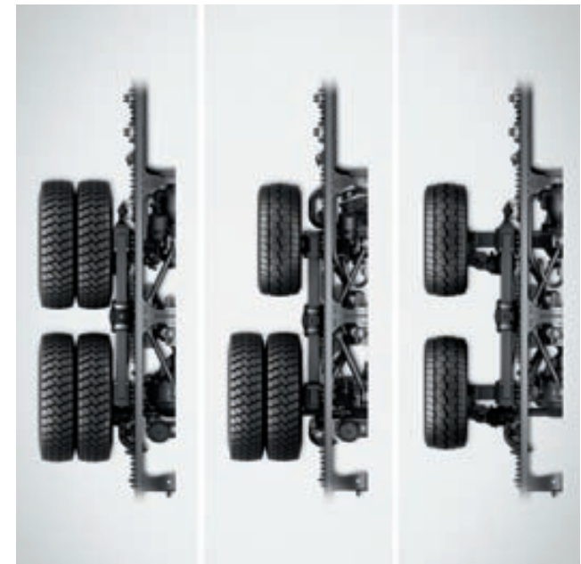
Payload-optimised tyre concepts. For transporting 8 m 3 of ready-mixed concrete the Arocs 8x4/4 concrete mixer is equipped with two widened hypoid rear axles for single tyres and particularly high-load-capacity 385/65 R22.5 wide-base tyres. As well as the payload gained, the low consumption also boosts efficiency
