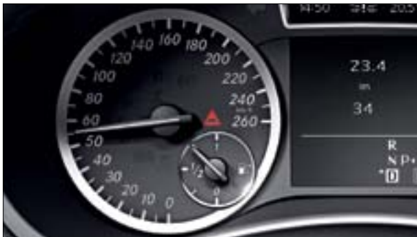
Collision Prevention Assist alerts the driver via acoustic and visual warning if the distance to the car in front becomes too low.
