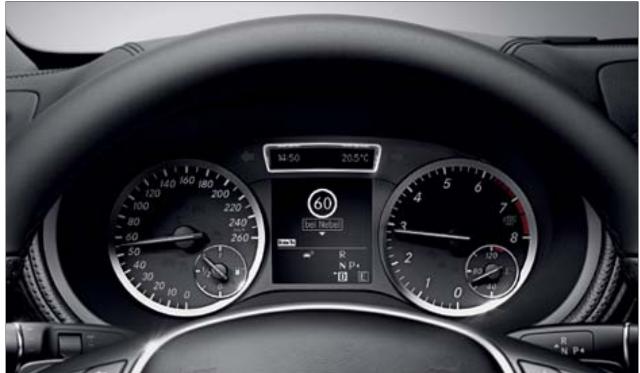
The Speed Limit Assist alerts the driver to the current speed limit
