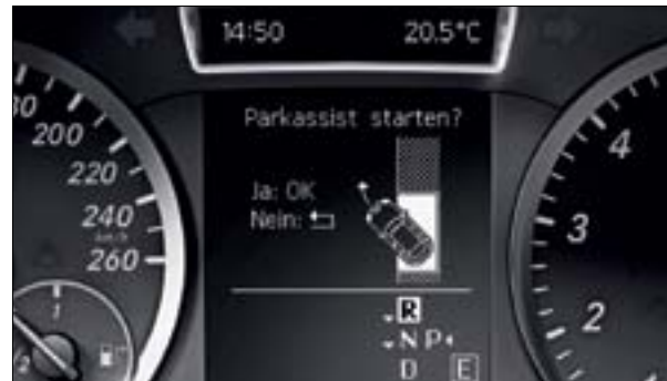
The multifunction display informs the driver about the current parking process
