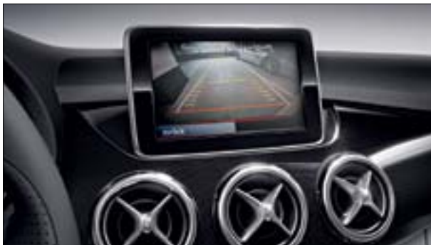
The central display shows the area behind the car during a parking manoeuvre
