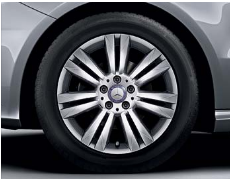
Optional for B-Class SE: 17" 7-twin-spoke alloy wheels, tyre size 225/45 R17 (code 26R)
