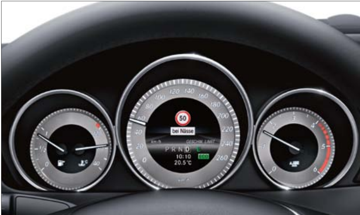
Speed Limit Assist even recognises and displays temporary speed restrictions
