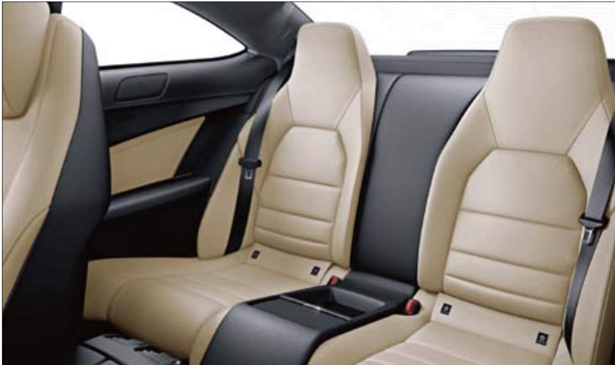
The standard Easy-Entry system facilitates access to the rear, sliding the front seats all the way forward when released
