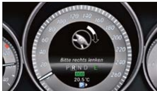
At speeds of up to 22 mph, Advanced Parking Guidance can automatically measure the length of parallel parking spaces
