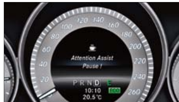
Attention Assist can detect the onset of tiredness and alert you to the need for a break
