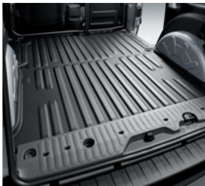
● Synthetic floor covering for passenger and load compartment 1 . This sound-absorbing synthetic floor covering is easy to clean and protects the floor against scratches and dents
