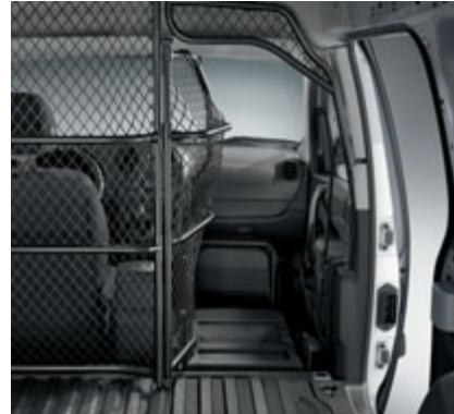
○ Foldable front passenger seat and cargo retention grille 1 . This creates a flat surface and a larger passenger compartment of up to 2886 mm, depending on vehicle length
