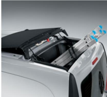
○ Ladder flap. The ladder flap at the rear of the roof allows long items to be transported
