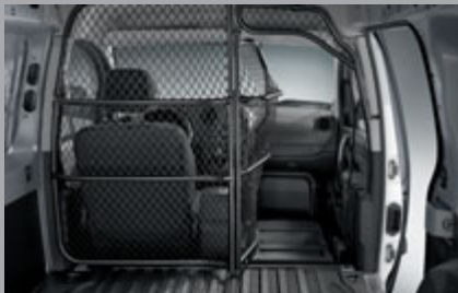
Folding Bulkhead. The panel van's optional folding grille bulkhead allows the loading length to be extended, and it helps protect the occupants
