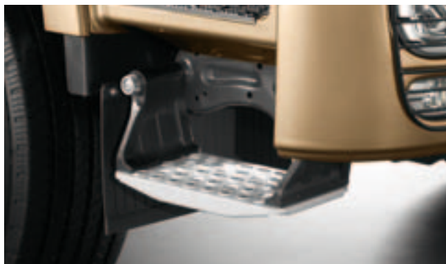
On tippers, concrete mixers and all-wheel-drive vehicles, the pivoting access step 2) is secured to the truck by rubber elements. If this step is struck by a boulder, or touches the ground, for example, it recoils in both a longitudinal and a transversal direction, thus providing protection against damage
