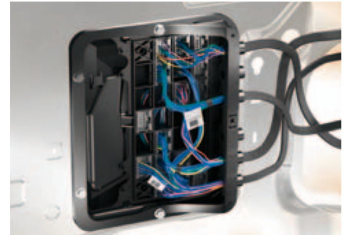
The bodybuilder interface allows bodybuilders easy, uncomplicated access to the Atego's electrical systems. This saves time and costs and makes for easier "communication" between the vehicle and body
