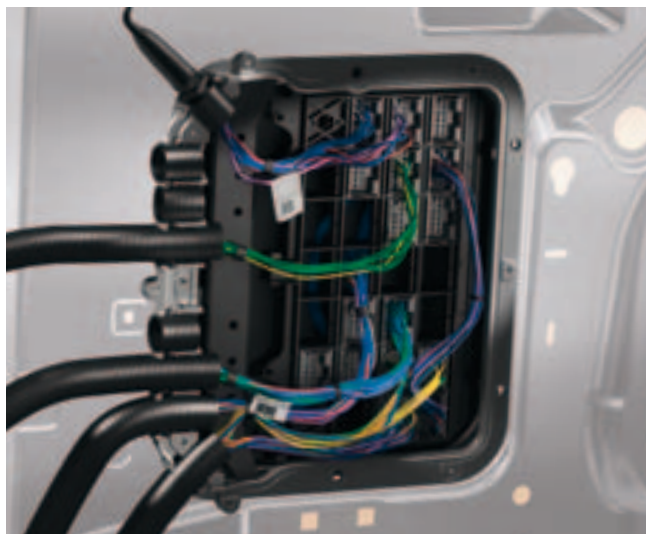
The parameterisable special module (PSM) is an interface for bodybuilders. It enables data exchange between the vehicle electronics and attachments, as well as the external control of vehicle functions
