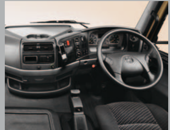
The dimensions of the standard-specification “Distribution” cockpit are such that it enables extremely convenient through-cab access in conjunction with the short engine tunnel of the 4-cylinder engines, while still featuring plenty of handy stowage space
