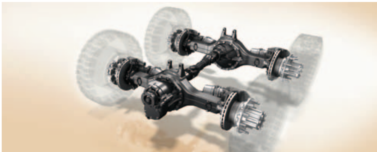
The low-maintenance, robust HL 4 hypoid rear axle is installed on 4-axle trucks in conjunction with the HD 4 through-drive axle as a tandem-axle assembly. Now produced using metal forming technology, the axle has a lower unladen weight, and a greater load-bearing capacity
