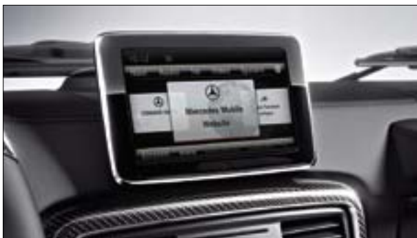
COMAND Online combines in-car entertainment, hard disk drive navigation and a high-resolution 7-inch central display
