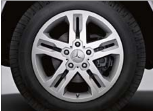
18" 5-twin-spoke alloy wheels with 265/60 R18 tyres (standard on G350 BlueTEC, code RM9)
