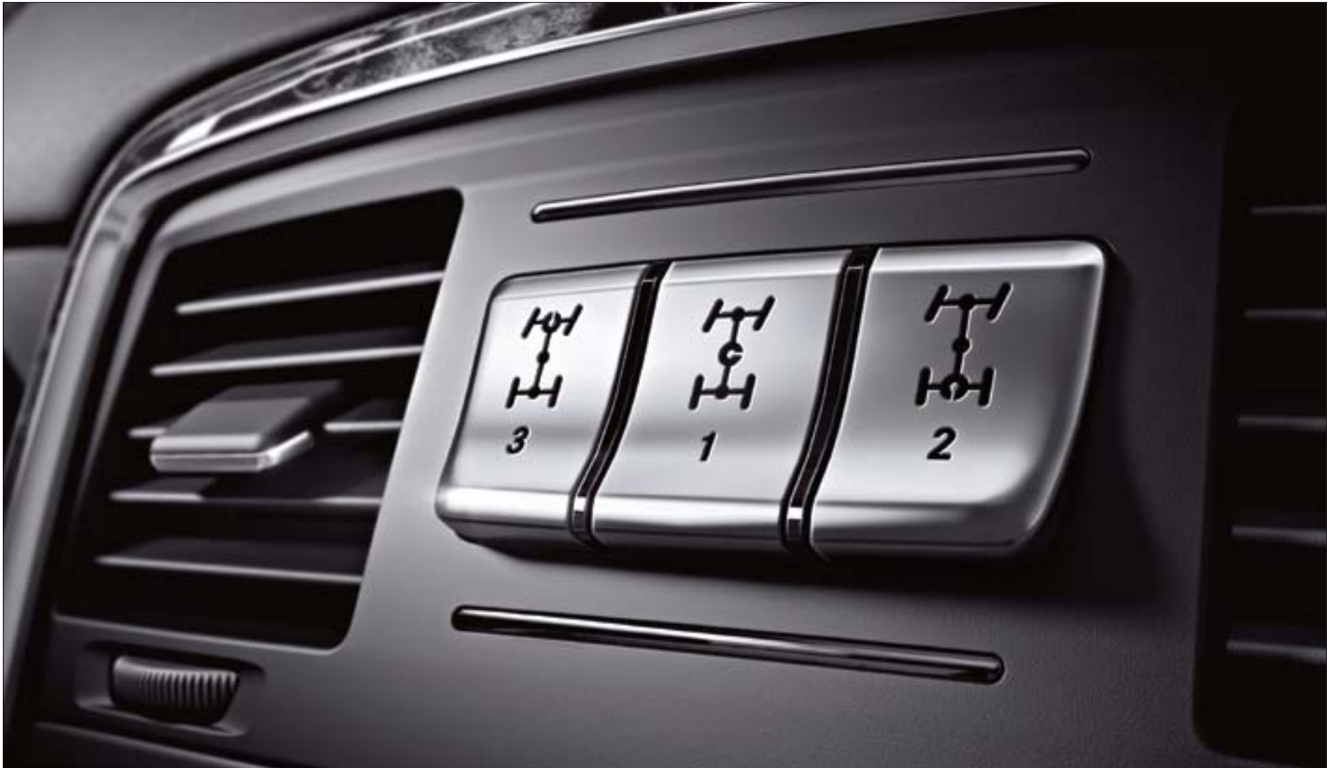
Three sequentially lockable differentials help the G-Class to overcome even the toughest off-road situations
