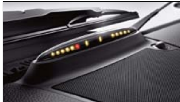
Parktronic's LEDs indicate the distance from other objects when manoeuvring
