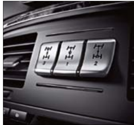
Sequentially lockable differentials
